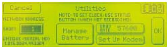
The Utilities screen allows for battery management and configuration of communication requirements.
