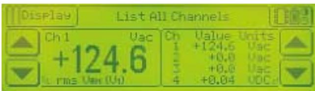
Users can scroll through all channels to view real-time values in two independent panels.
