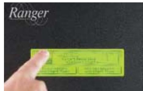
Pressing the upper left corner of the screen accesses the Menu Flow feature, which shows users exactly where they are in the menu sequence.
